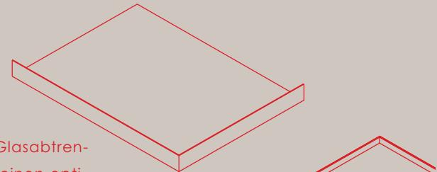
**Roof „Top“.** Our steam bath tops optimally top-off the installation, ensuring that the steam cannot escape. They can be placed onto the steam bath or hidden almost entirely from view behind the shower enclosure.
