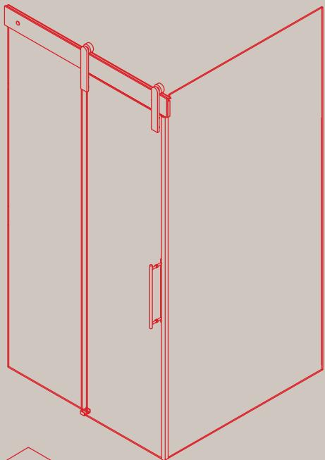
**Steam door shower enclosure.** Made to measure, it ensures that the steam cannot escape out of the cubicle, resulting in strong steam formation within the cubicle. It also provides spray protection when showering.
